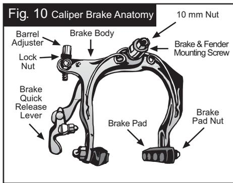
**Fig. 10** Caliper Brake Anatomy
