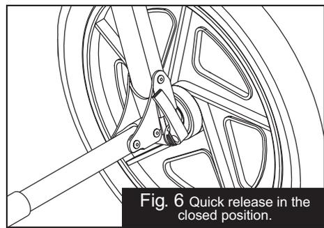
**Fig. 6** Quick release in the closed position.
