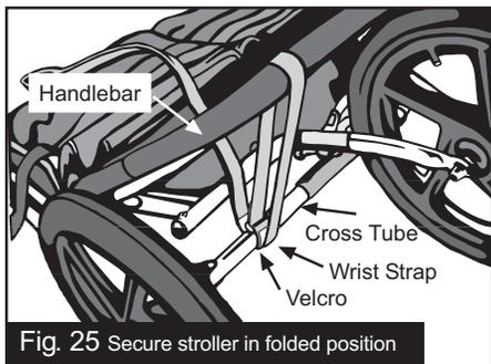
Fig. 25 Secure stroller in folded position
