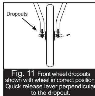
**Fig. 11** Front wheel dropouts shown with wheel in correct position. Quick release lever perpendicular to the dropout.
