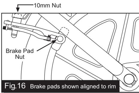
Fig. 16 Brake pads shown aligned to rim
