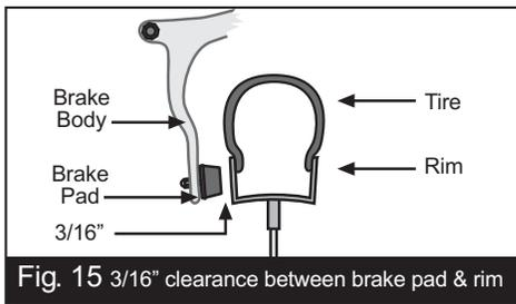
Fig. 15 3/16" clearance between brake pad & rim
