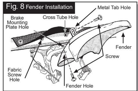
**Fig. 8** Fender Installation
