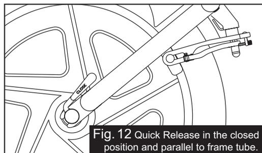
**Fig. 12** Quick Release in the closed position and parallel to frame tube.
