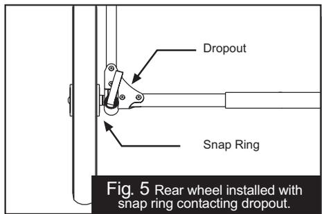
**Fig. 5** Rear wheel installed with snap ring contacting dropout.
