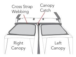
**3. Secure Canopy Catch** Hold Canopy Catch in place and tighten screw with screwdriver.
