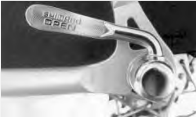
FIG. 24 Bicycle quick release in open position.
