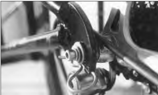
FIG. 37 Derailleur side pin rotated perpendicular to outside face of trailer hook.
