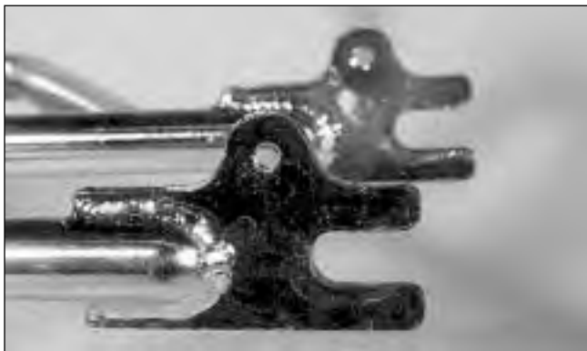
FIG. 13 Slotted rear dropout for axle insertion.
