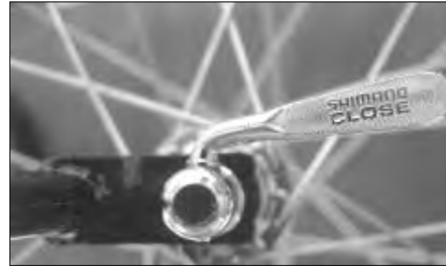
FIG. 16 Quick release in closed position.
