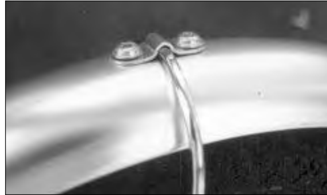
FIG. 9 Attach the fender bracket to the fender with mounting hardware as shown.
