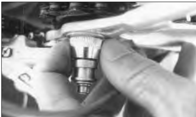
FIG. 30 Adjusting approximately 1.5mm dropout.
