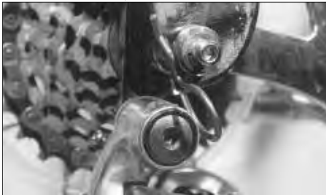
FIG. 4 Trailer in extreme clockwise rotation showing contact between derailleur mount and retaining pin. AVOID this condition. If you believe this has occurred, inspect your derailleur, QR, and pins for damage
