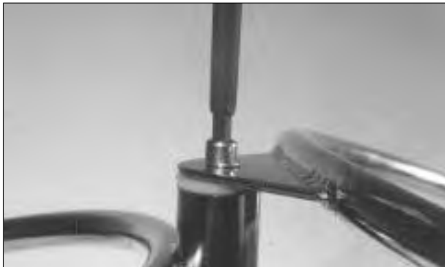
FIG. 22 Tighten YAK front fork pivot screws in the upper and lower pivot.
