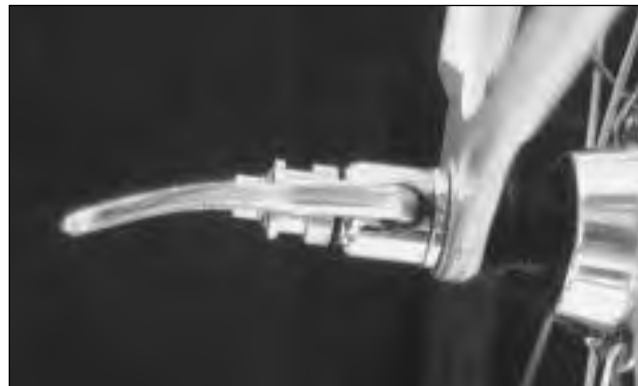
FIG. 29 Quick release perpendicular to the frame.
