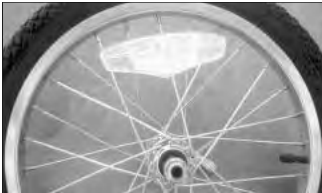
FIG. 17 Wheel reflector correctly positioned.
