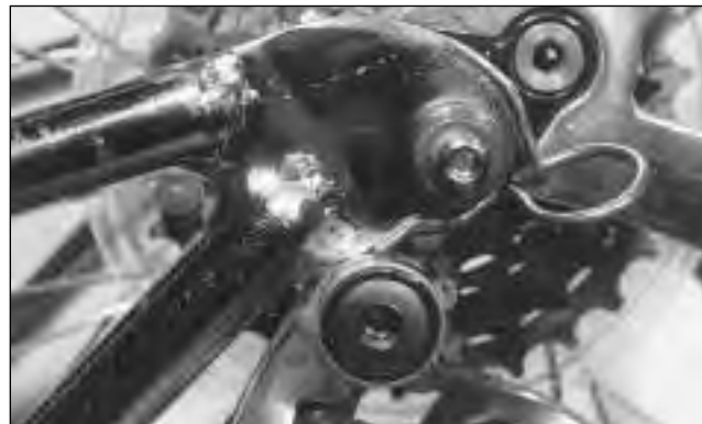
FIG. 3 Trailer in extreme counter-clockwise rotation showing contact between derailleur pivot housing and trailer fork. AVOID this condition. If you believe this has occurred, inspect your derailleur, QR, and pins for damage. Note: reversing the installation of the QR (install from the drive side / right side of bike) helps eliminate this problem ( Fig. 5a ).
