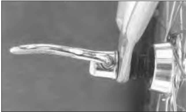
FIG. 15 Quick release perpendicular to the trailer
