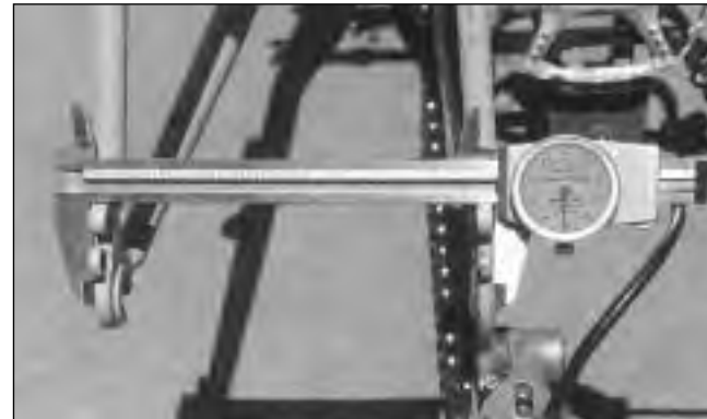
FIG. 25 Measurement of outside to outside dimension of rear dropouts.
