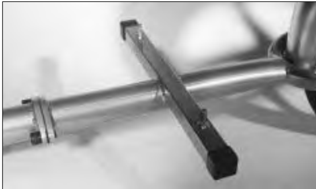
FIG. 6 Flanges of "boom tube" and COZ flange bolts.
