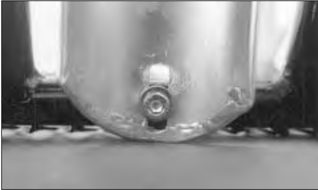
FIG. 10 Attachment of fender to trailer frame.
