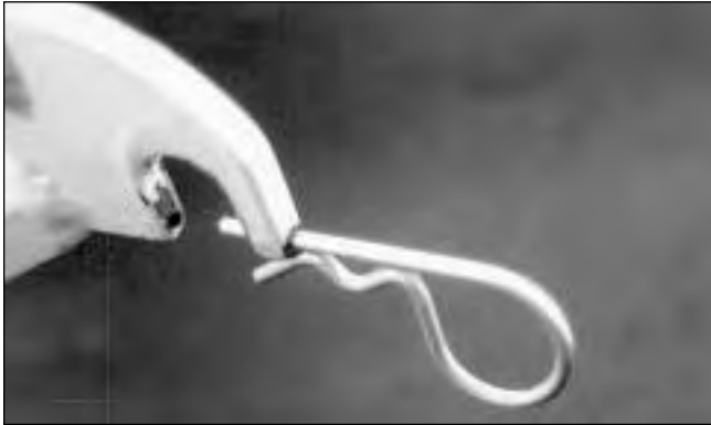
FIG. 35 Pin insertion hole in front edge of hook.
