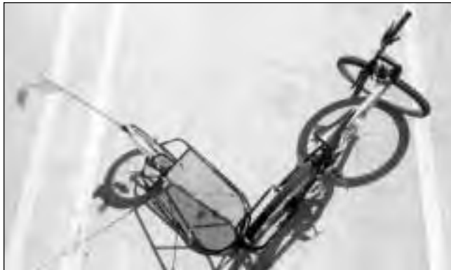
FIG. 5 Correct way to park bike and trailer. Note: correct direction to turn the handlebars is towards the trailer. Trailer and handlebars are 90 degrees to bike.
