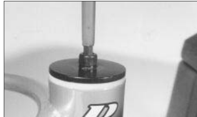
FIG. 21 Tighten COZ front fork pivot screw in the upper and lower pivot.
