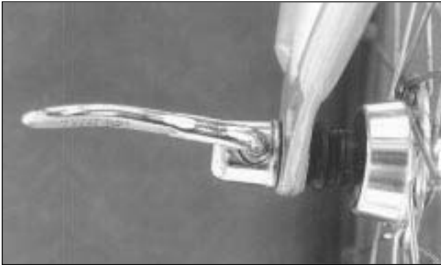
FIG. 15 Quick release perpendicular to the trailer
