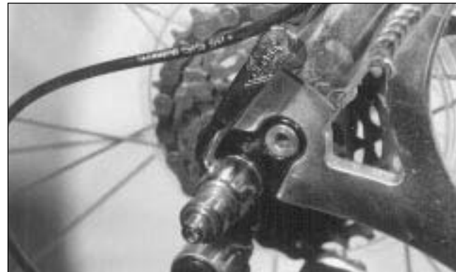
FIG. 5a B.O.B QR installed from drive side/right side of bike.
