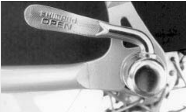
FIG. 24 Bicycle quick release in open position.
