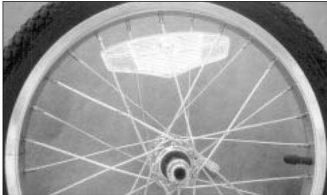
FIG. 17 Wheel reflector correctly positioned.
