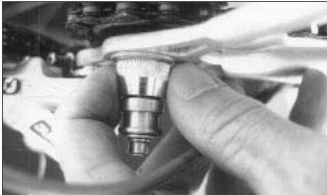
FIG. 30 Adjusting approximately 1.5mm dropout.
