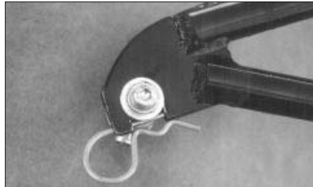
FIG. 36 Retention pin correctly inserted into hook so top edge of second loop rests in hook slot.
