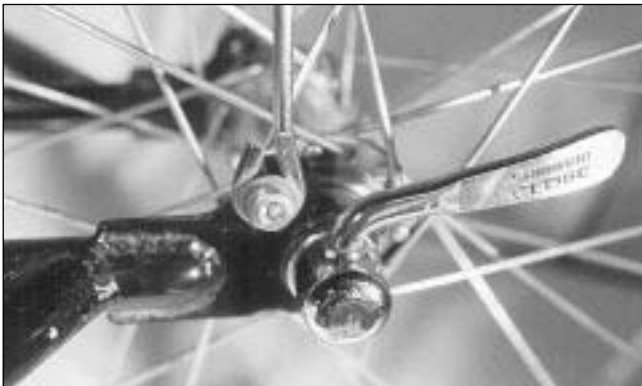
FIG. 11 Attachment of the fender to the dropout eyelet.
