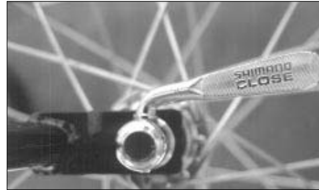
FIG. 16 Quick release in closed position.
