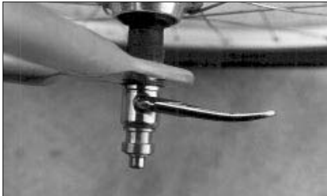
FIG. 26 Correct orientation of quick release in rear wheel.
